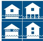
**Elevation** is raising your home so that the lowest floor is above the flood level. This is the most common way to avoid flood damage.
