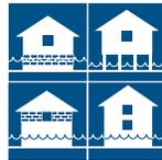
For example, this series of illustrations from the guide shows how a home on a basement or crawlspace foundation can be elevated above the flood level on extended foundation walls.
